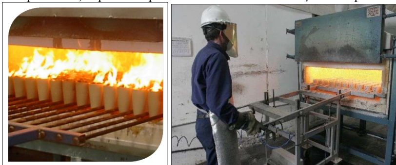
Fig. 1. Încărcarea creuzetelor în cuptorul de fuziune ( https://www.alsglobal.com/-/media/als/resources/services-and-products/geochemistry/technical-notes/fire-assay-technical-note-2012.pdf , https://alexstewartinternational.com/portfolio-item/19-fire-assay-loading-furnace/ )
